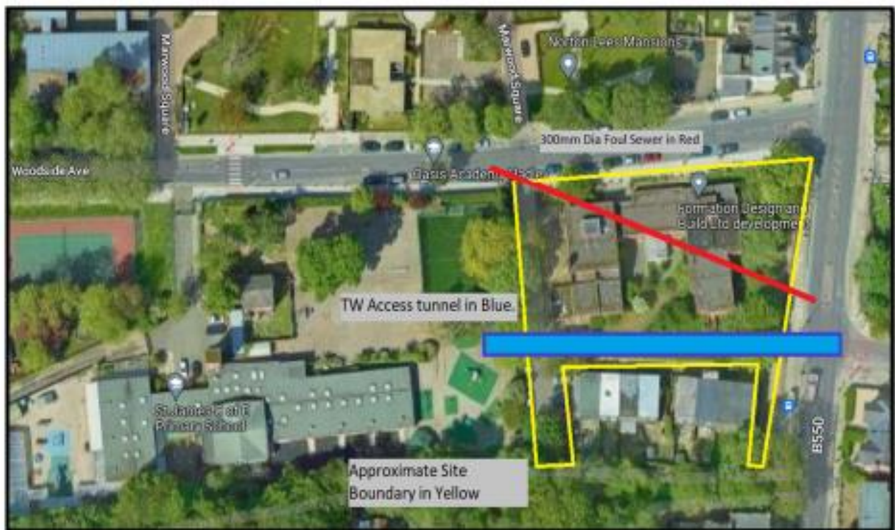
Figure 1 Aerial View of Site indicating TW Assets. Cranwood House (yet to be demolished) can be seen to have been built over the 300mm diameter Foul water sewer.
