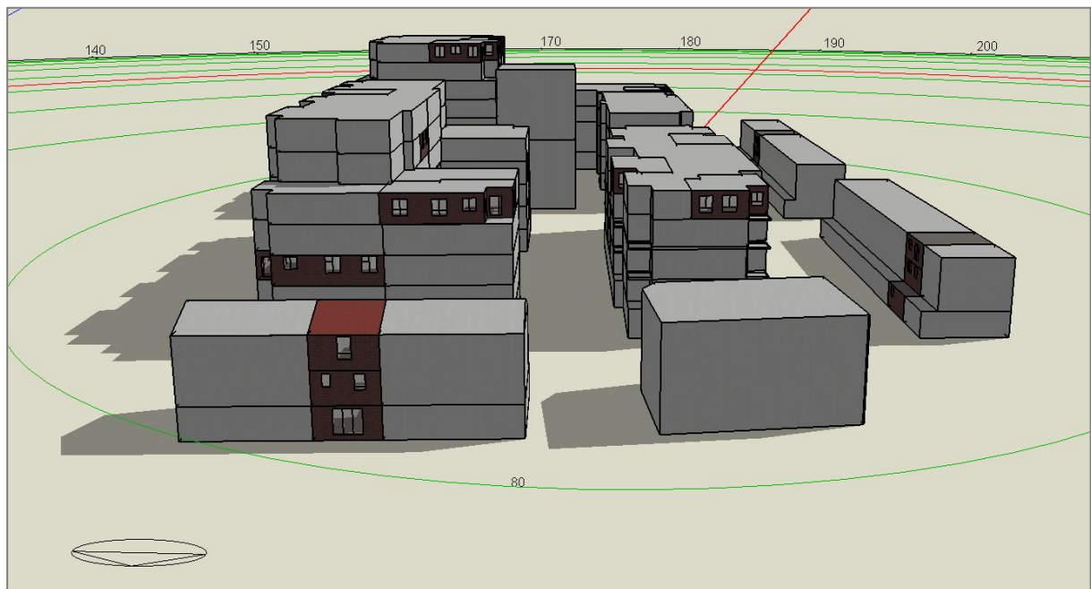
Figure 5: Building simulation model from Design Builder Software, viewed from the north, with shadows generated from sun path diagram for 21 June 15:00
