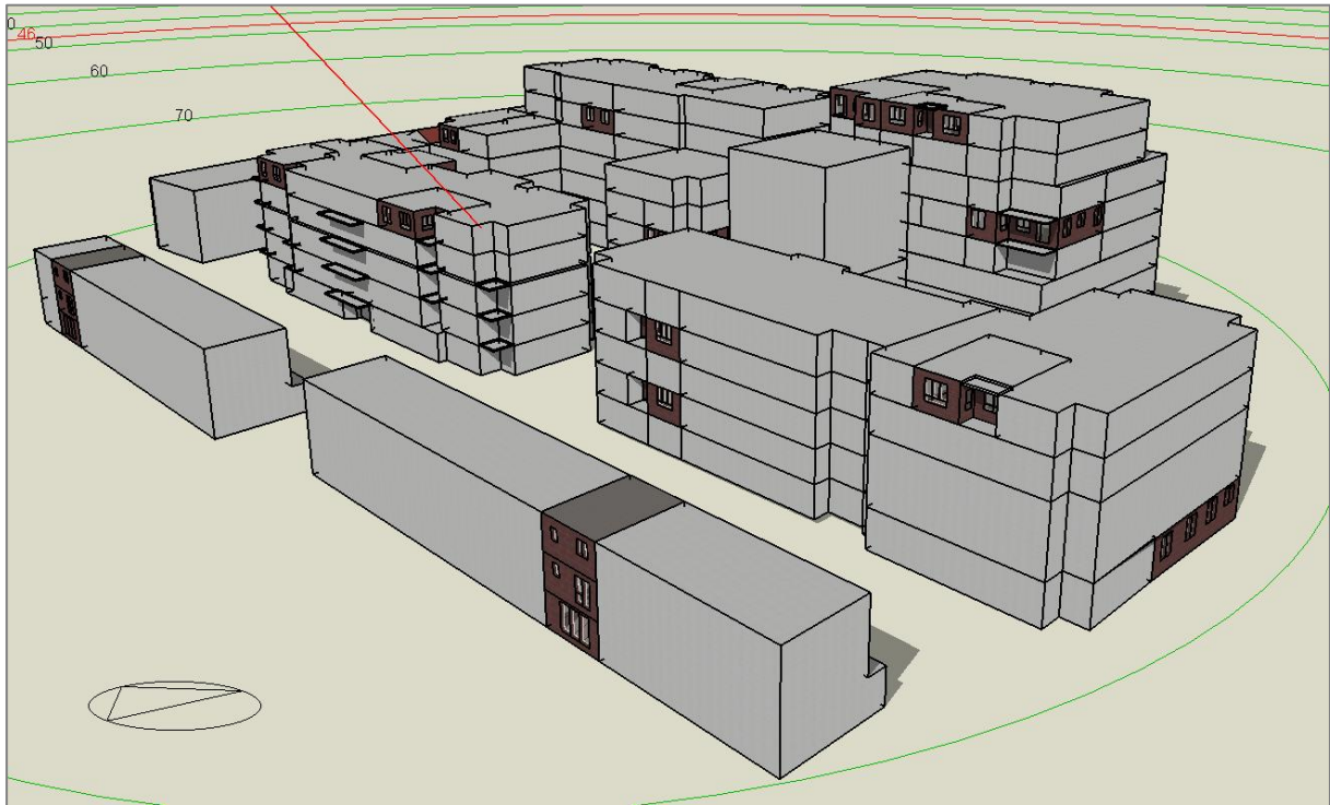
Figure 6: Building simulation model from Design Builder Software, viewed from the south west, with shadows generated from sun path diagram for 21 June 15:00
