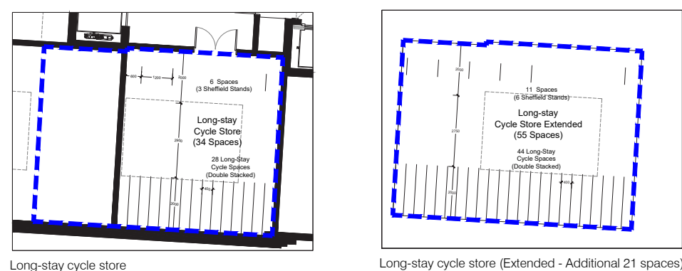
FIGURE 15 - RELOCATED CYCLE STORE AND FUTURE EXTENDABILITY
