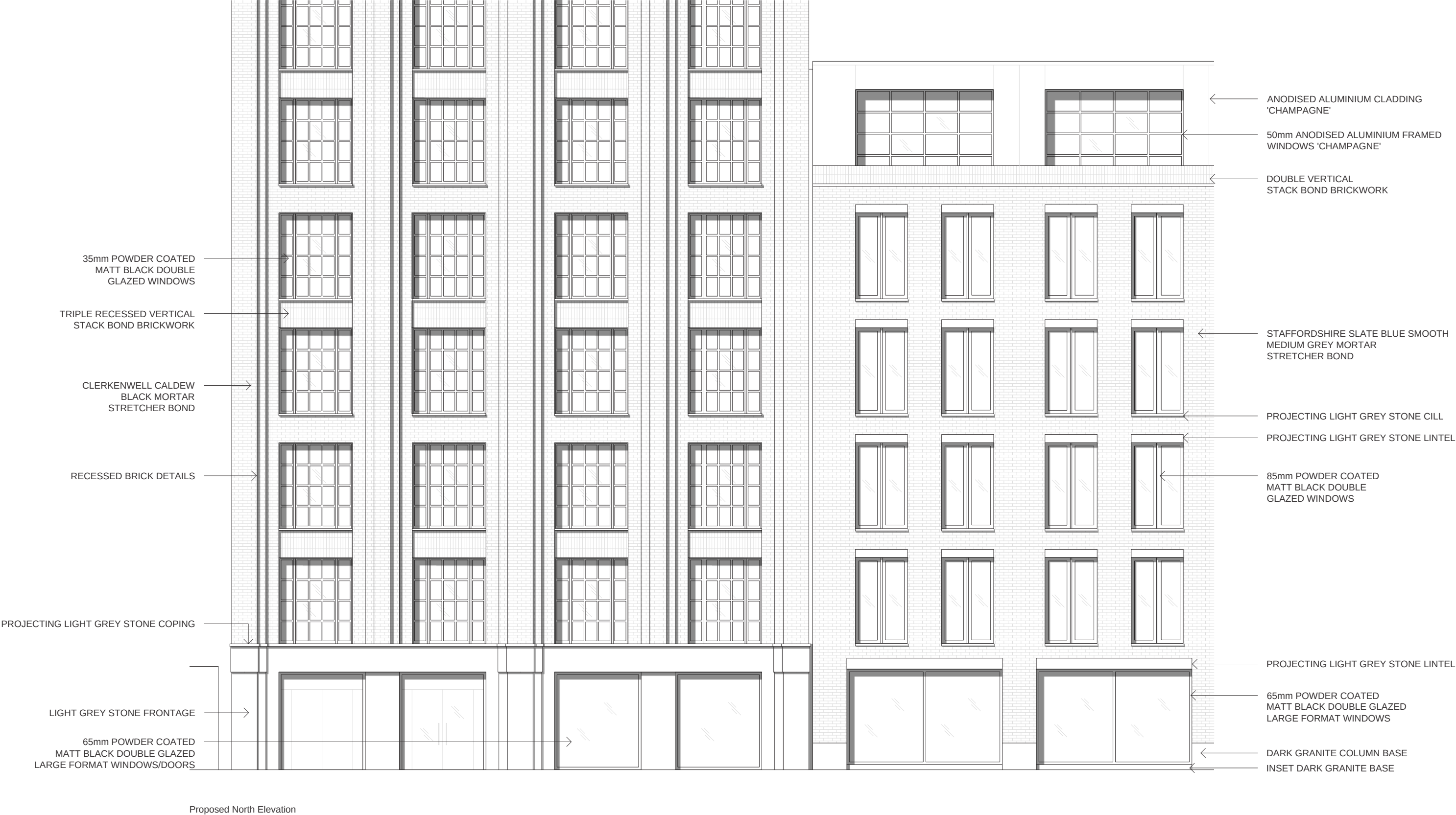
FIGURE 20 - PROPOSED LONG ELEVATION MATERIALS AND DETAILING (PARTIAL)
