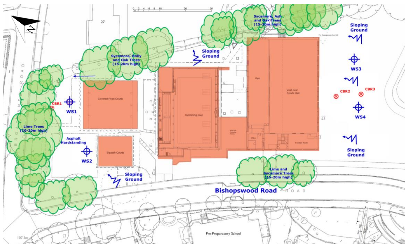
Figure 6.2 Ground investigation locations from the supplementary phase
