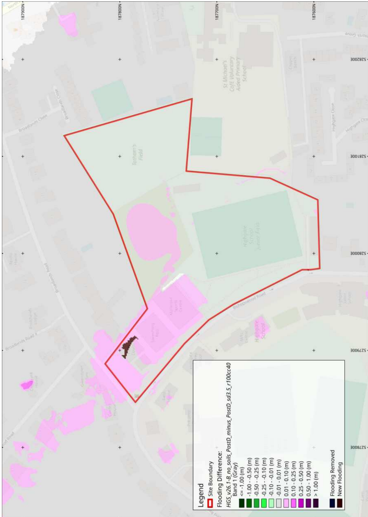
Figure 5.20: Post development scenario, maximum food depths difference between the modelled scenario (with soils) and the frozen catchment (without soils) for the 1 in 100 year design event plus 40% climate change
