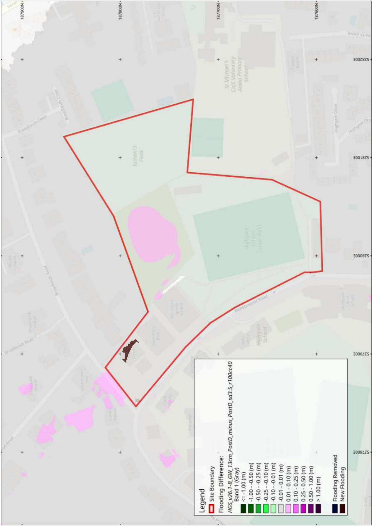
Figure G.4: Post development scenario, maximum food depths difference between the modelled scenario with the depth to groundwater of 25cm and the halved depth to groundwater of 13cm for the 1 in 100 year design event plus 40% climate change
