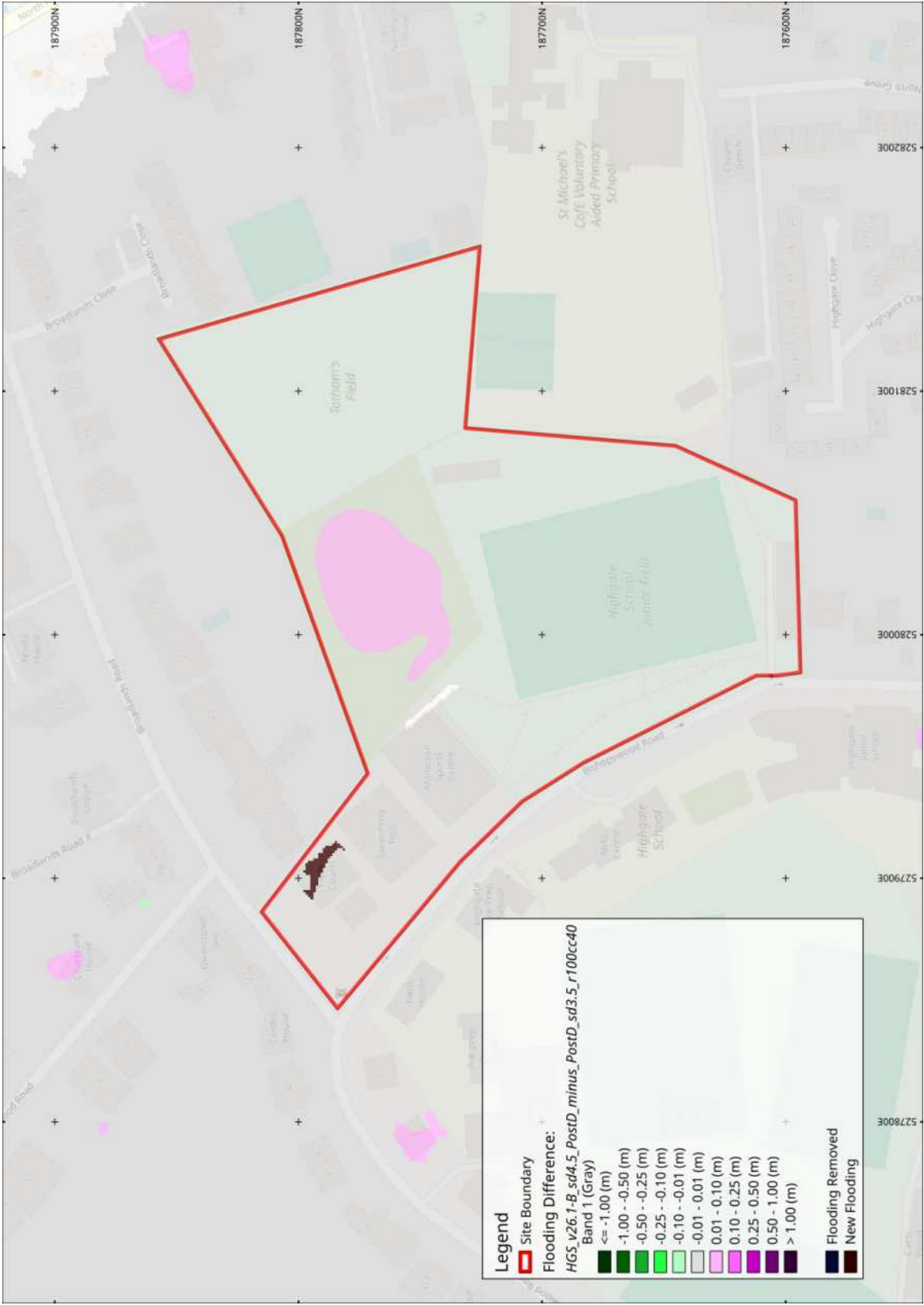
Figure G.1: Post development scenario, maximum food depths difference between the critical storm 3.5hrs and the 4.5hr storm duration for the 1 in 100 year design event plus 40% climate change
