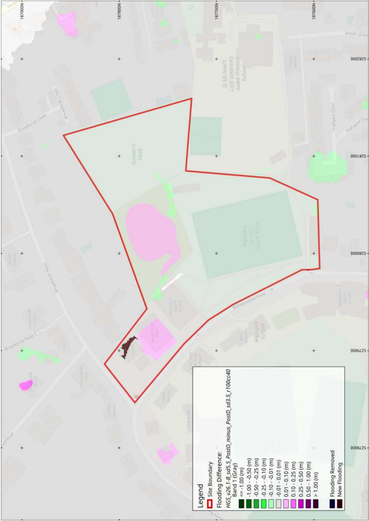
Figure G.2: Post development scenario, maximum food depths difference between the critical storm 3.5hrs and the 5.5hr storm duration for the 1 in 100 year design event plus 40% climate change
