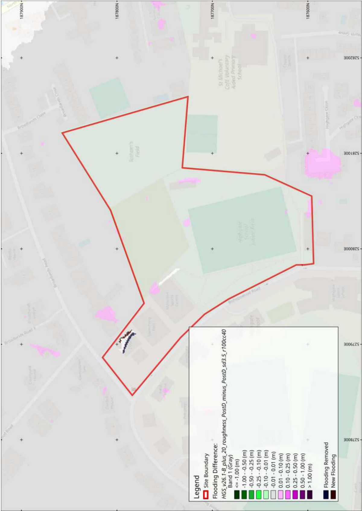
Figure G.6: Post development scenario, maximum food depths difference between the modelled scenario and a 20% increase in global roughness for the 1 in 100 year design event plus 40% climate change
