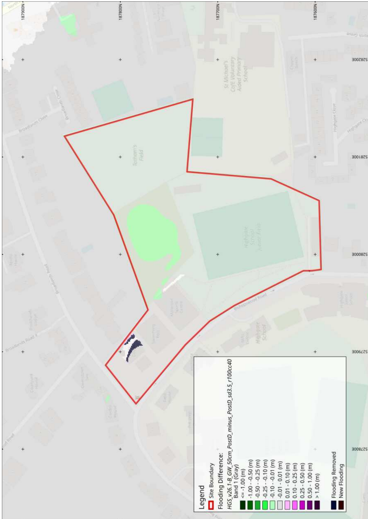
Figure G.5: Post development scenario, maximum food depths difference between the modelled scenario with the depth to groundwater of 25cm and the halved depth to groundwater of 50cm for the 1 in 100 year design event plus 40% climate change
