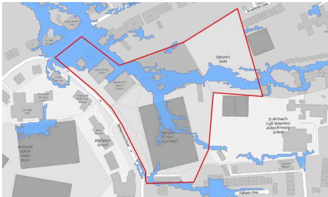
Figure 4.7: Surface Water Flood Risk (Low 0.1% AEP)
