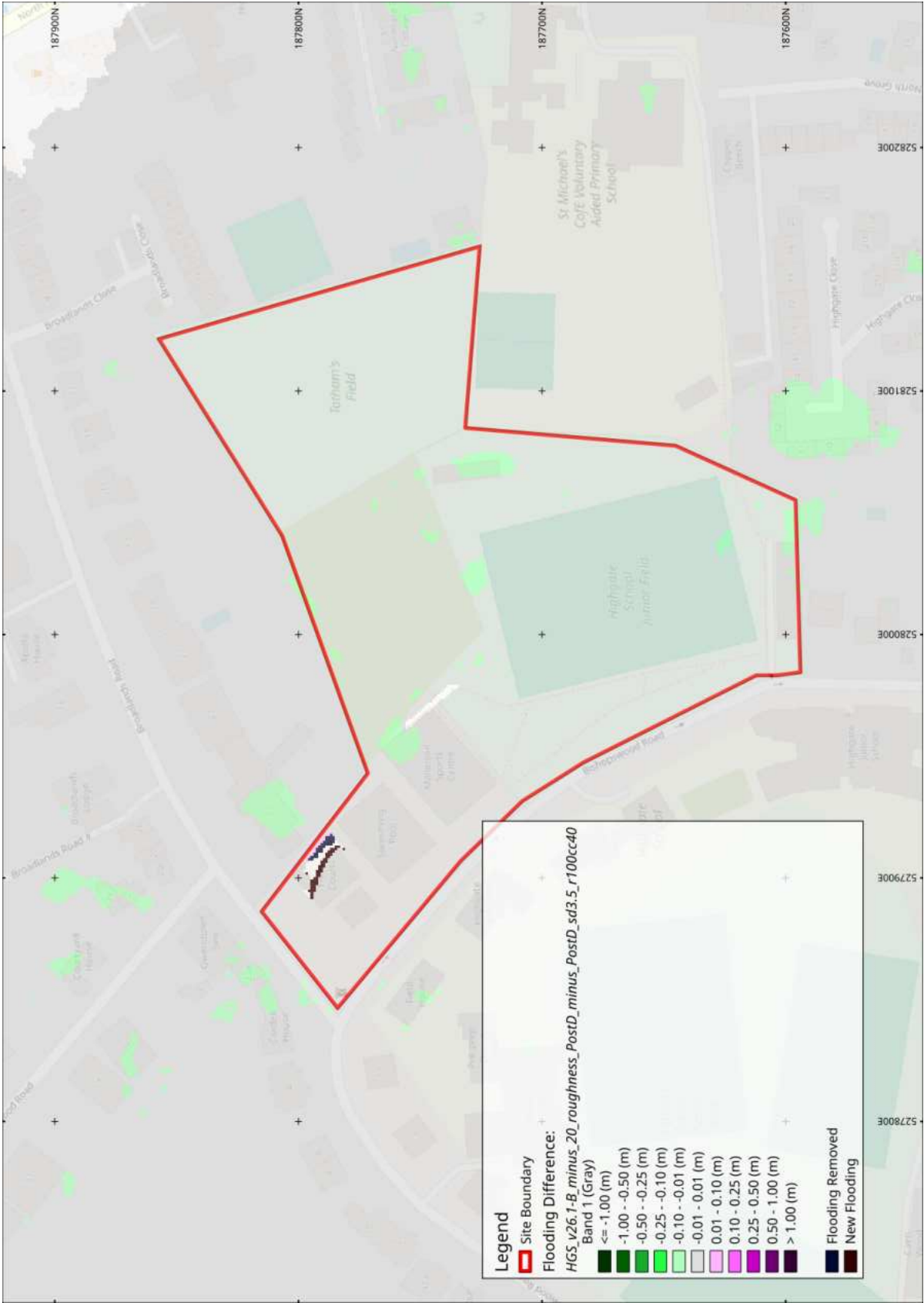
Figure G.7: Post development scenario, maximum food depths difference between the modelled scenario and a 20% decrease in global roughness for the 1 in 100 year design event plus 40% climate change
