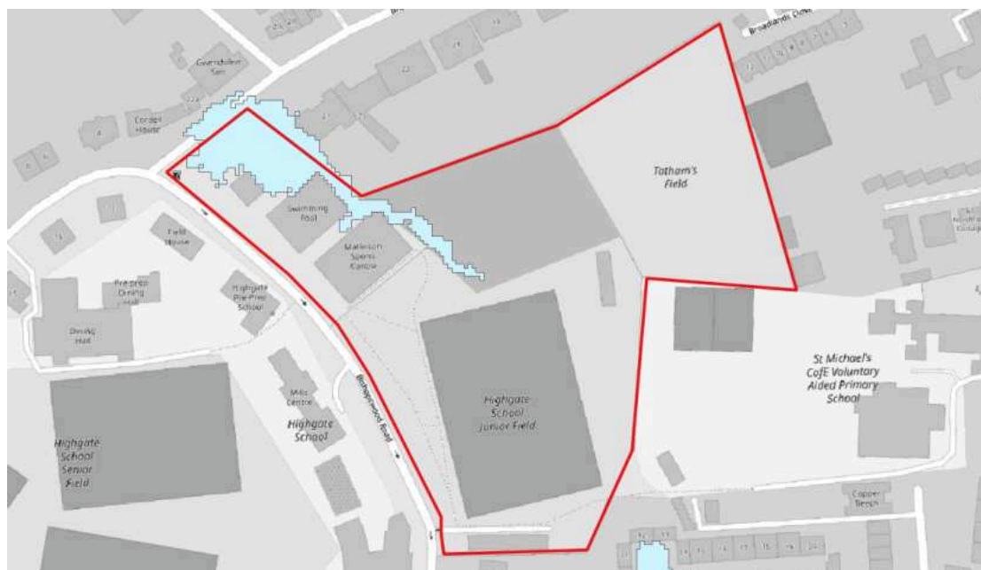
Figure 4.5: Surface Water Flood Risk (High 3.3% AEP)
