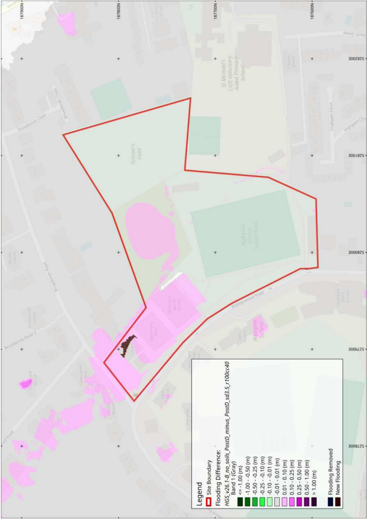
Figure G.3: Post development scenario, maximum food depths difference between the modelled scenario (with soils) and the frozen catchment (without soils) for the 1 in 100 year design event plus 40% climate change
