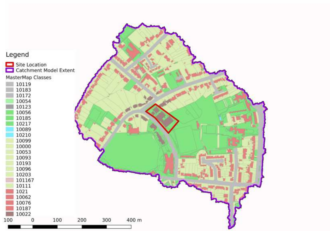
Figure 5.3: Coverage of different land-use classes to be assigned different roughness parameter values
