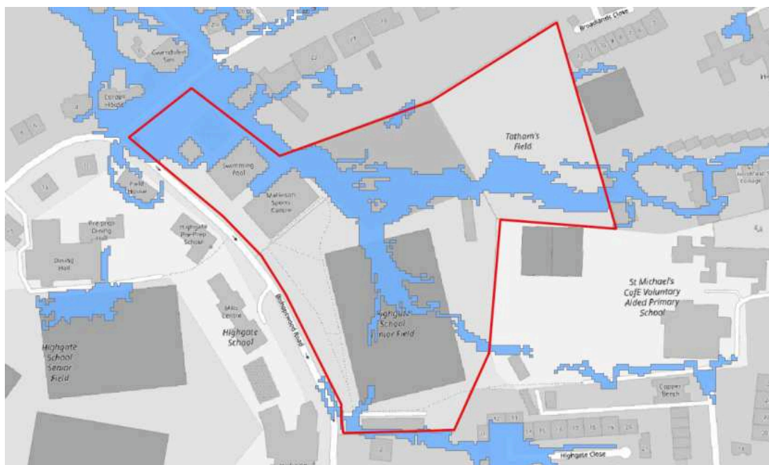
Figure 4.7: Surface Water Flood Risk (Low 0.1% AEP)
