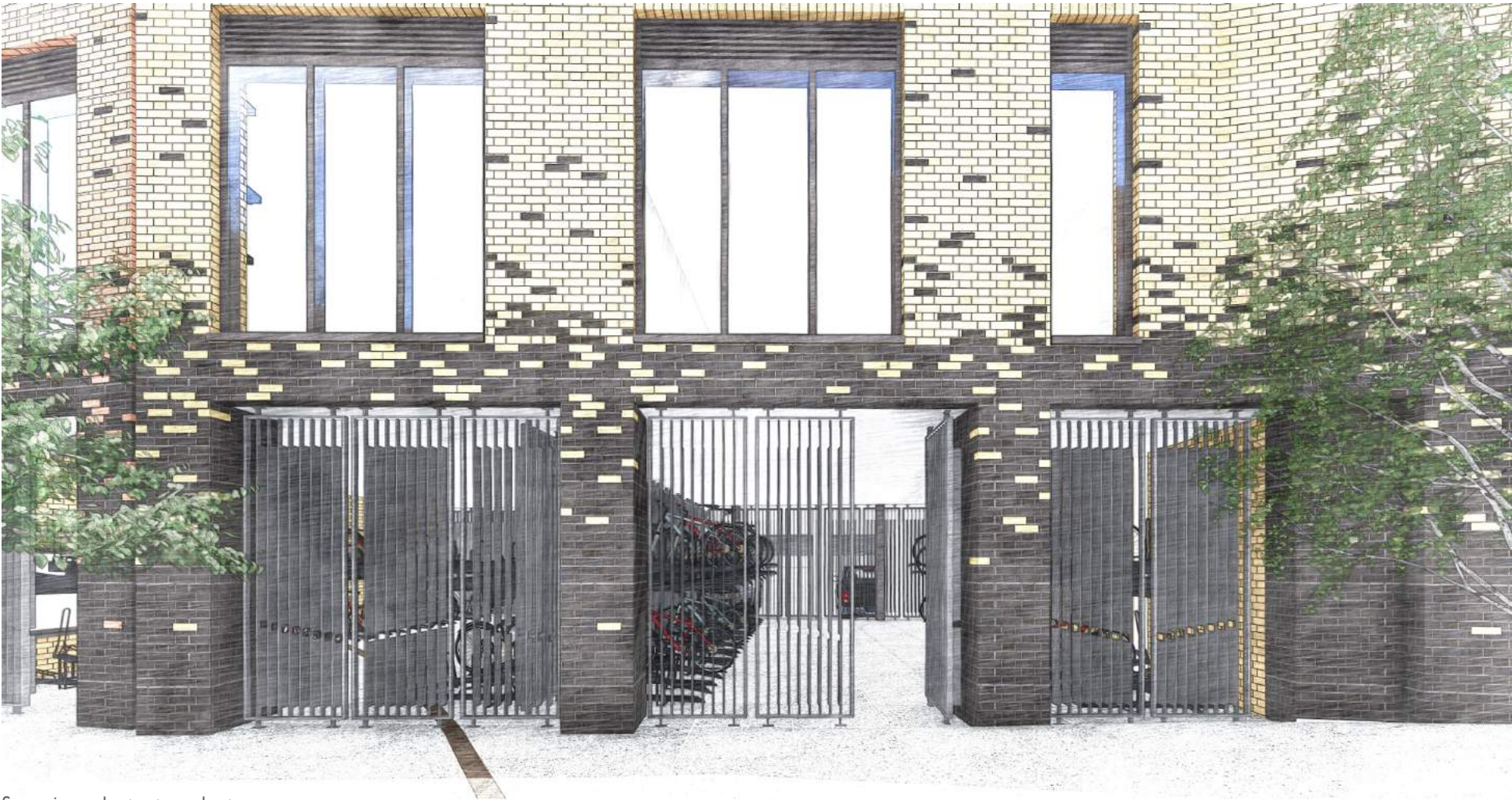
Screening and gates to cycle stores
