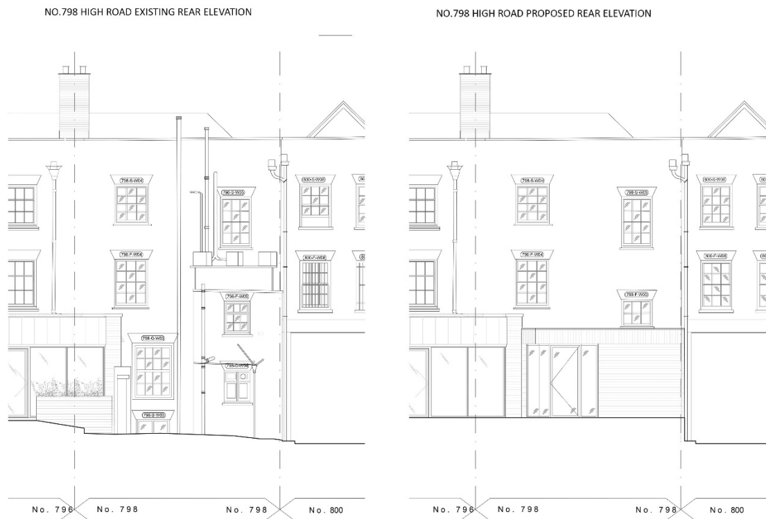
Figure 41: No.798 Existing and Proposed Rear Elevations
