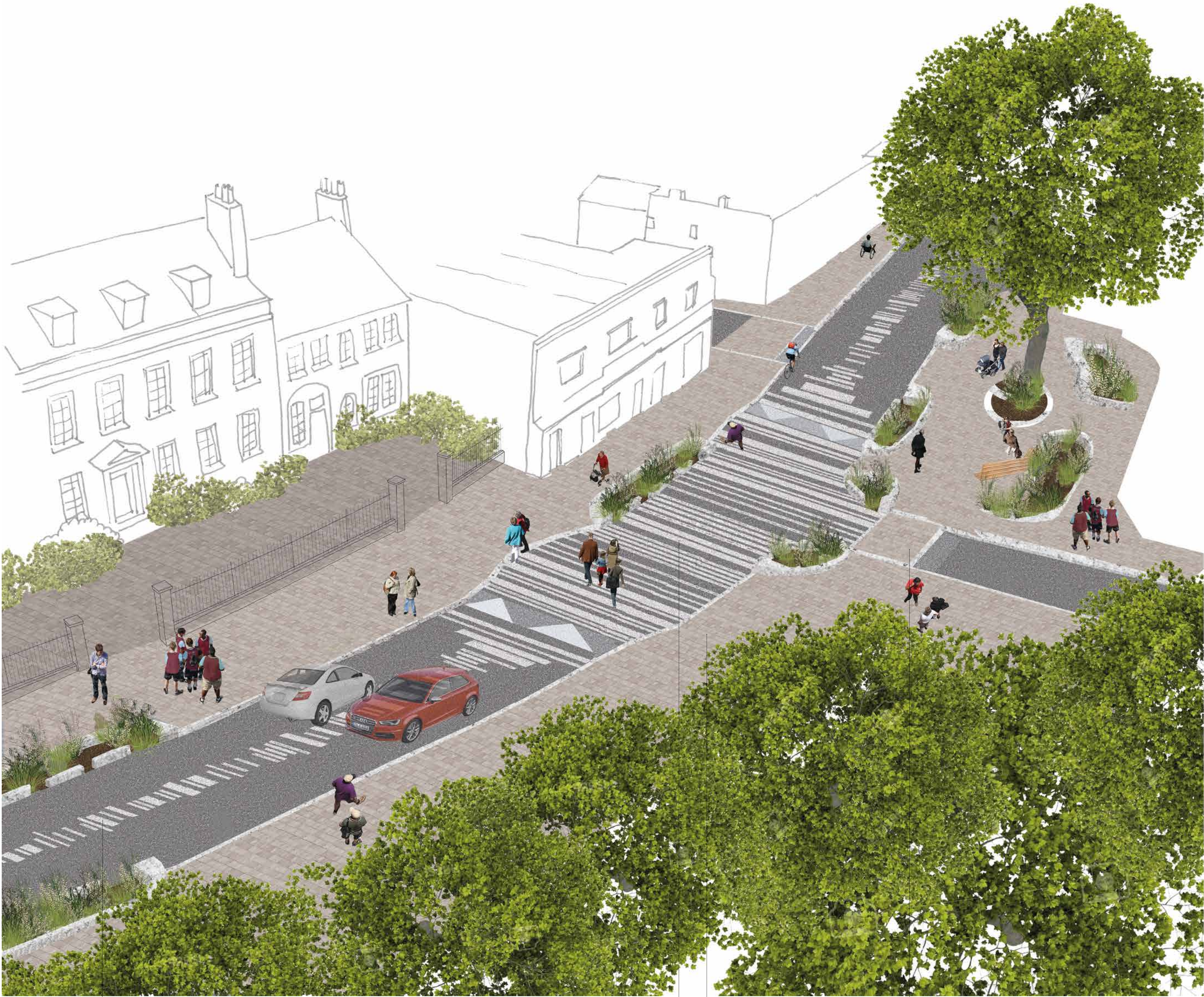
Central patterned strip to give the impression the road is narrower than it is
