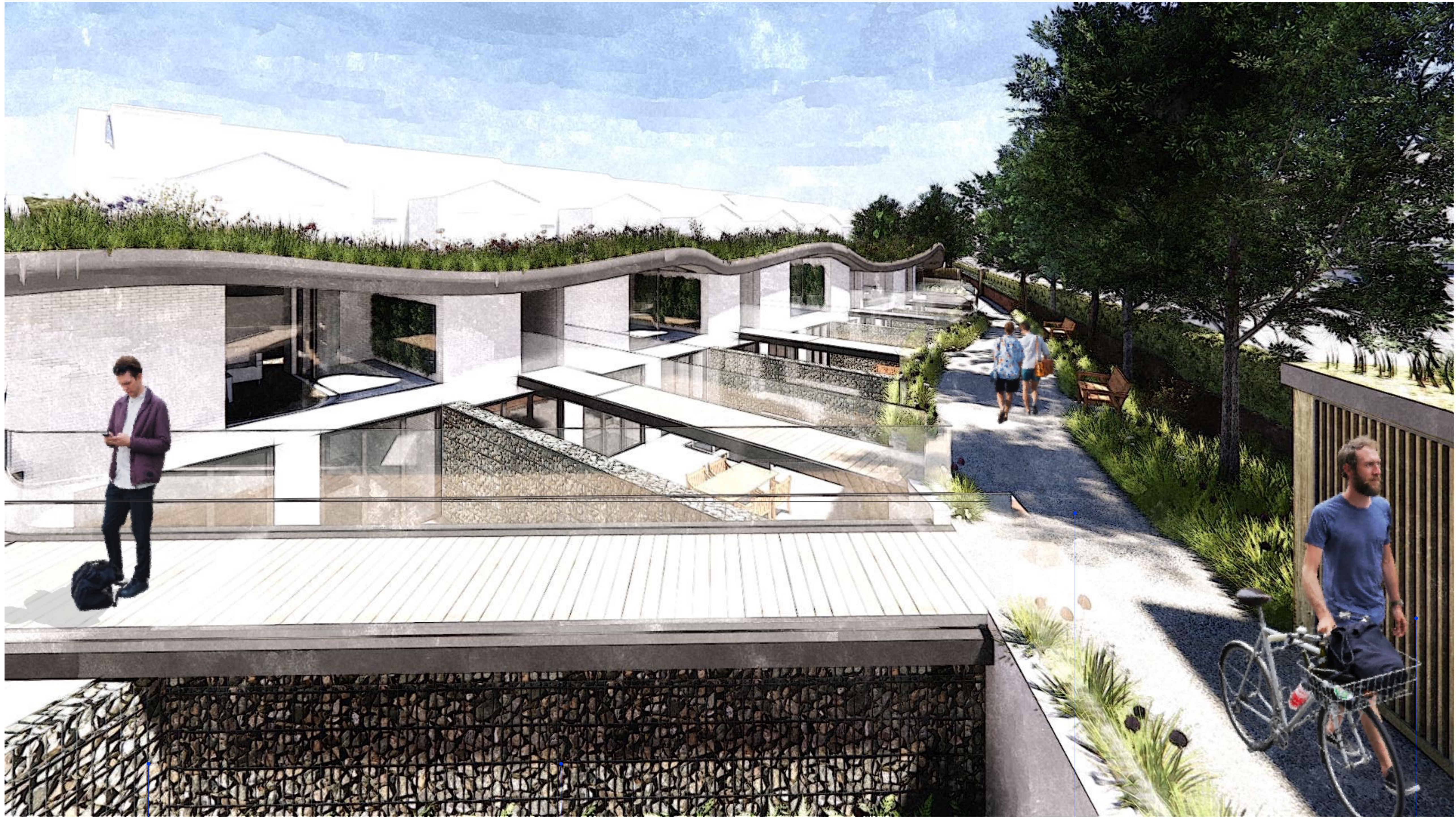
GABION WALLS SEPARATING LOW LEVEL TERRACES
