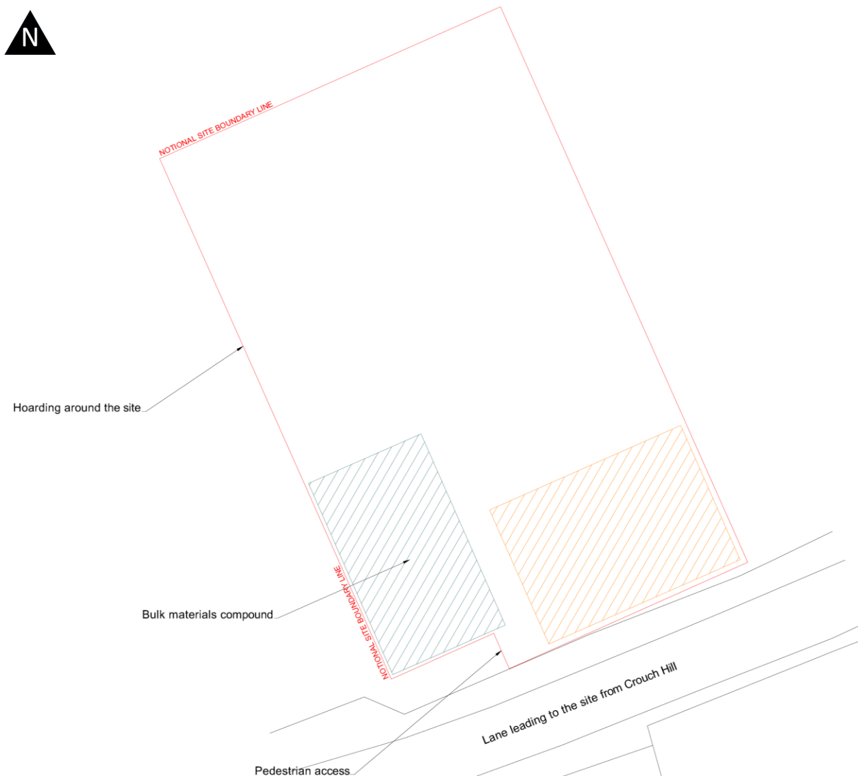
Figure 4.1 Construction site layout
