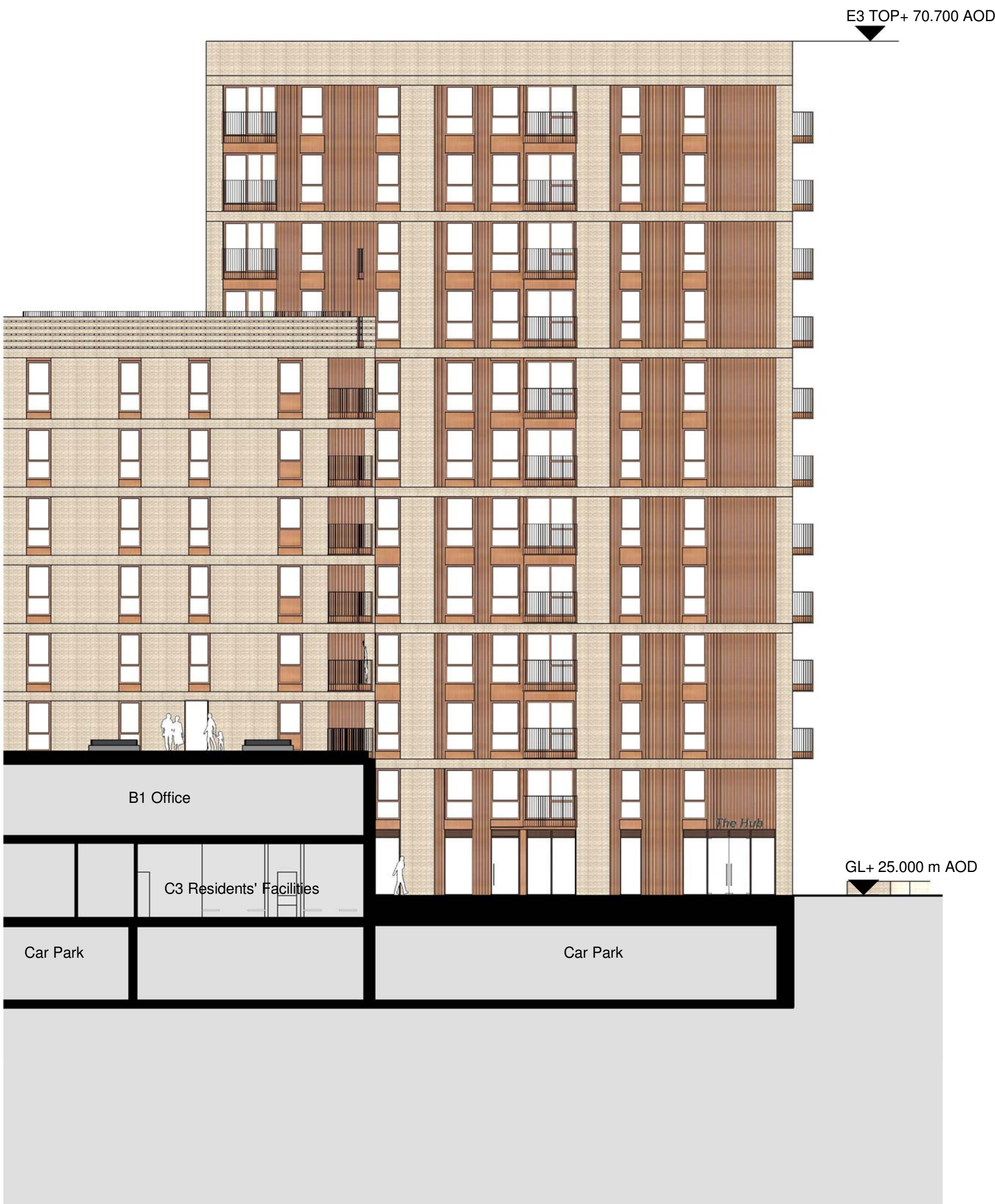
Block E1 - North Elevation EE
