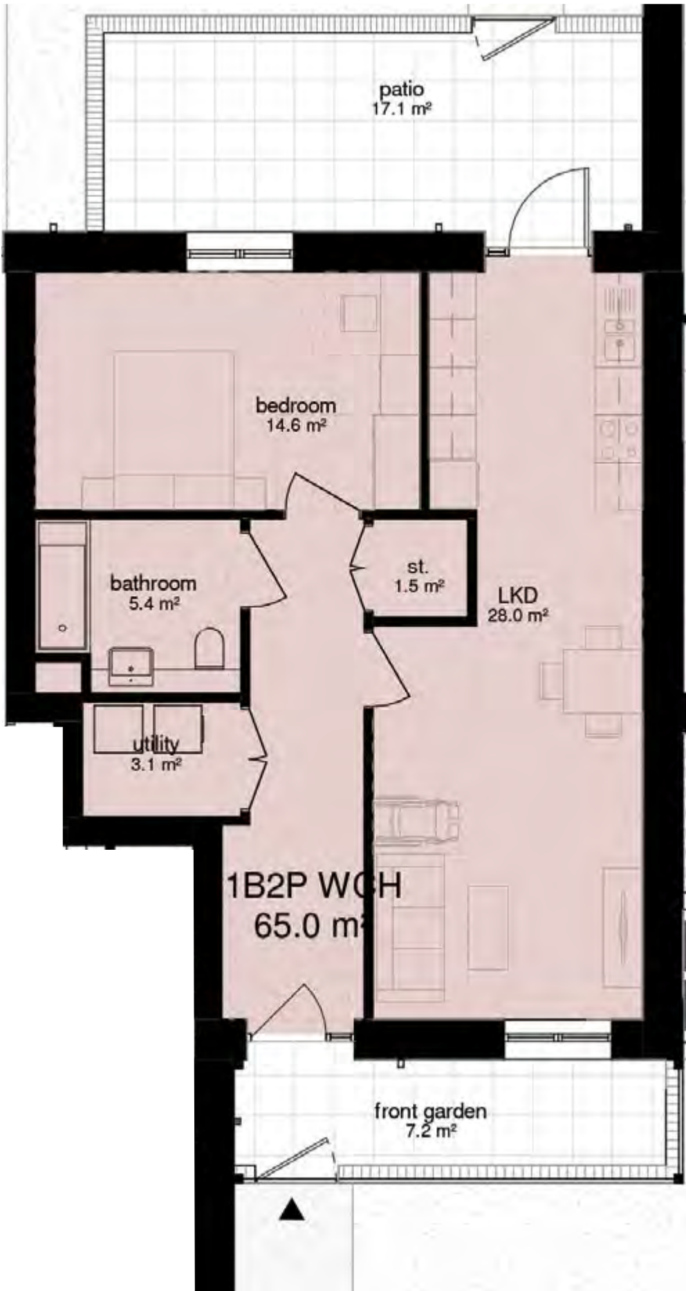
1B2P WCH Flat - Ground-floor plan
