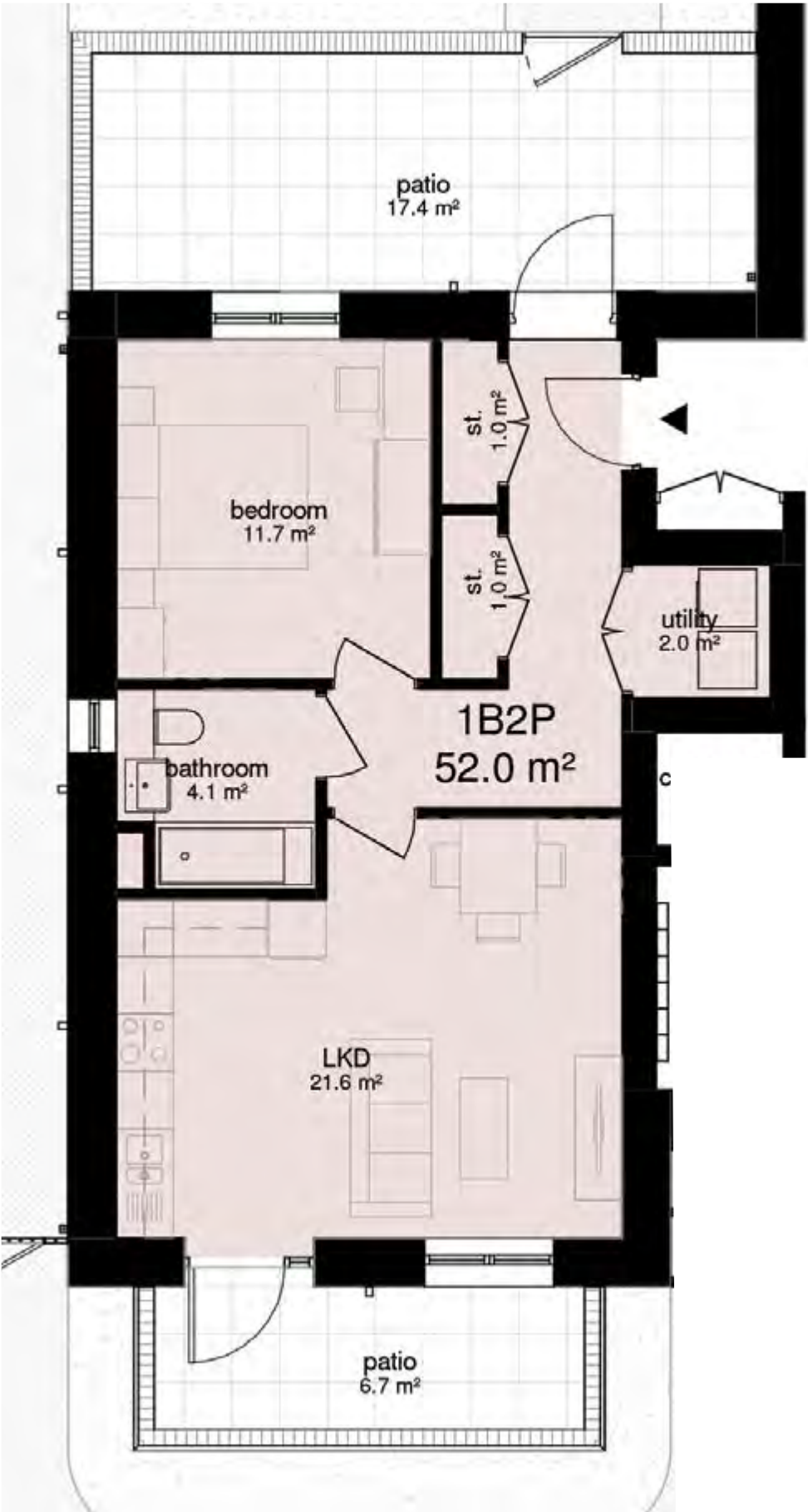
1B2P Flat - Ground-floor plan
