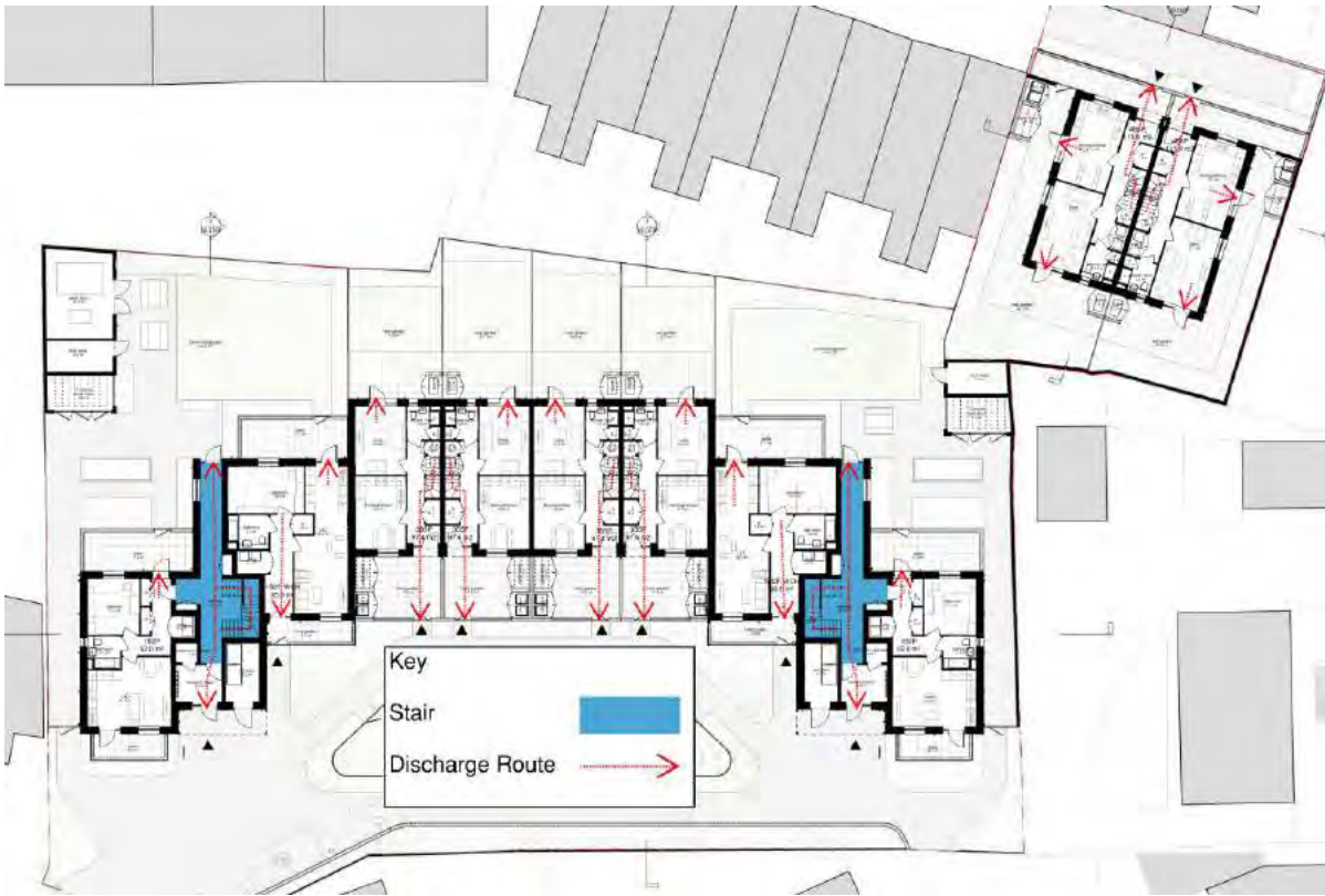
Figure 4: Final Discharge Route
