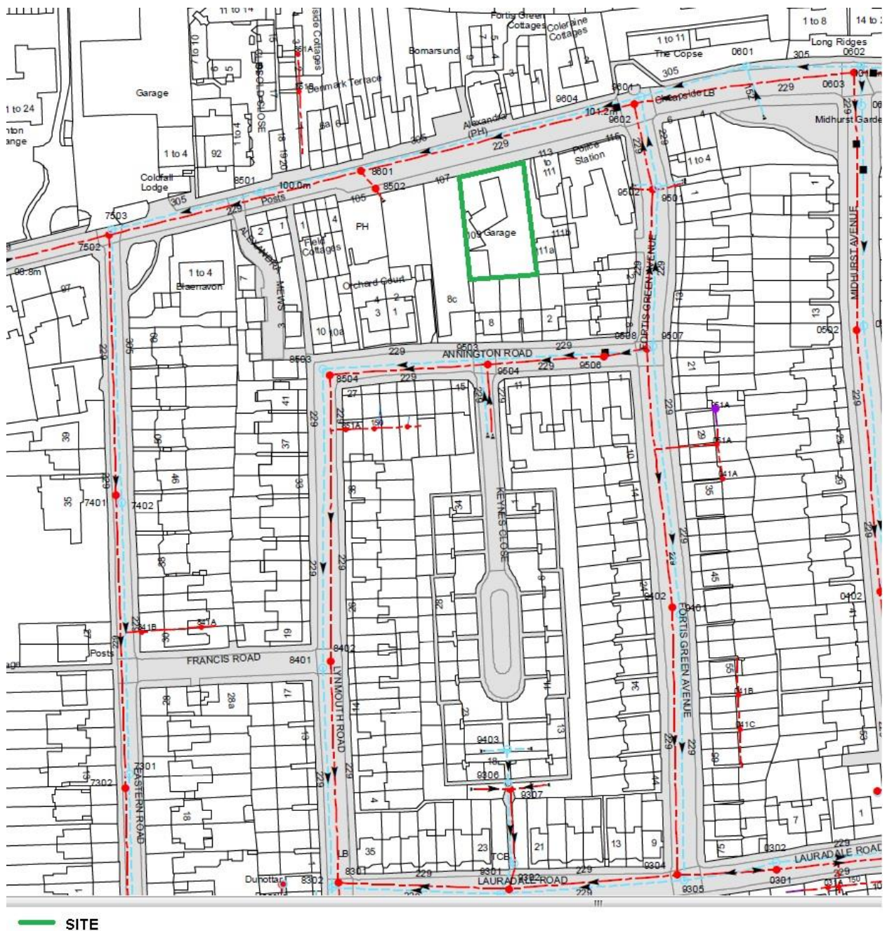
Figure 2.3: Thames Water Sewer Records
