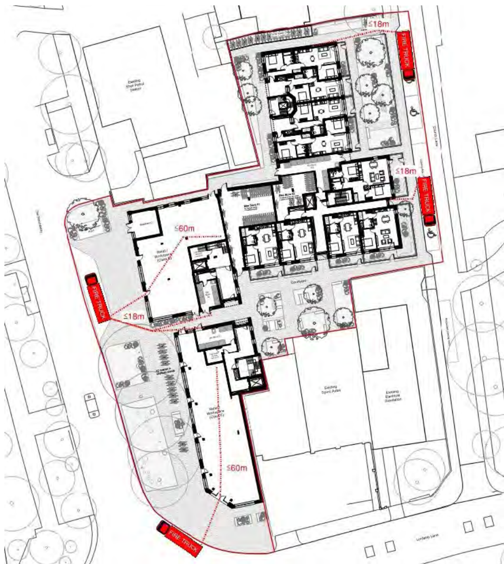
Fig. 142: Fire Strategy - Fire access to each block
