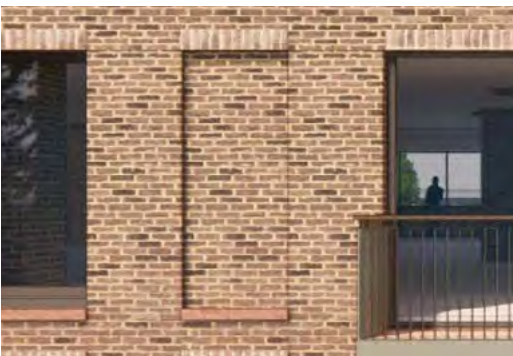
Blind window with terracotta sill and expressed lintel
