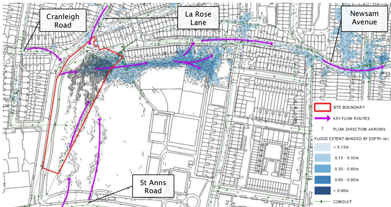
Figure 2-1: Flow Routes underlaid with 3.3% AEP Flood Extents
