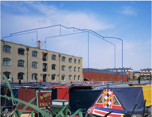
Example of AVR 1 confirming degree of visibility (in this case as an occluded ‘wire-line’ image)
