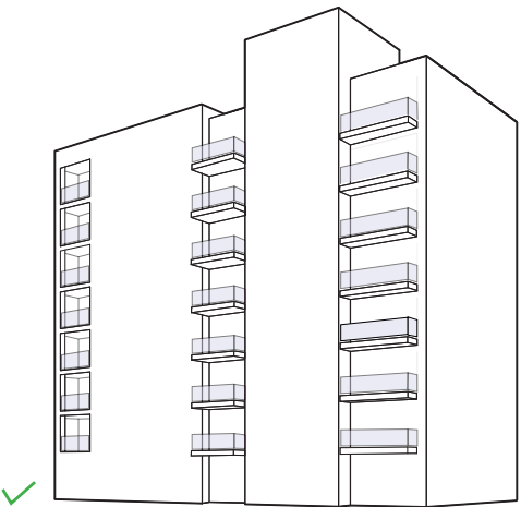
CODE D: Corner balconies can be enclosed with a column or exposed
