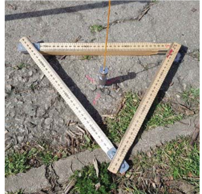
4: Survey reference point
