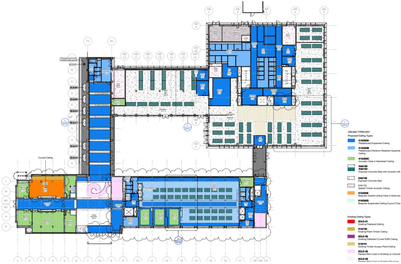
Figure 4-2 Ceiling layout for ground floor of project
