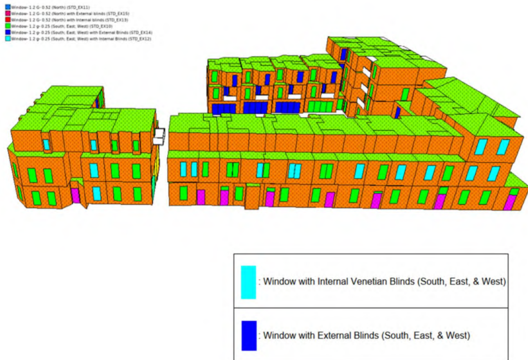
Figure 3.8: Venetian Blinds - (South Elevation)
