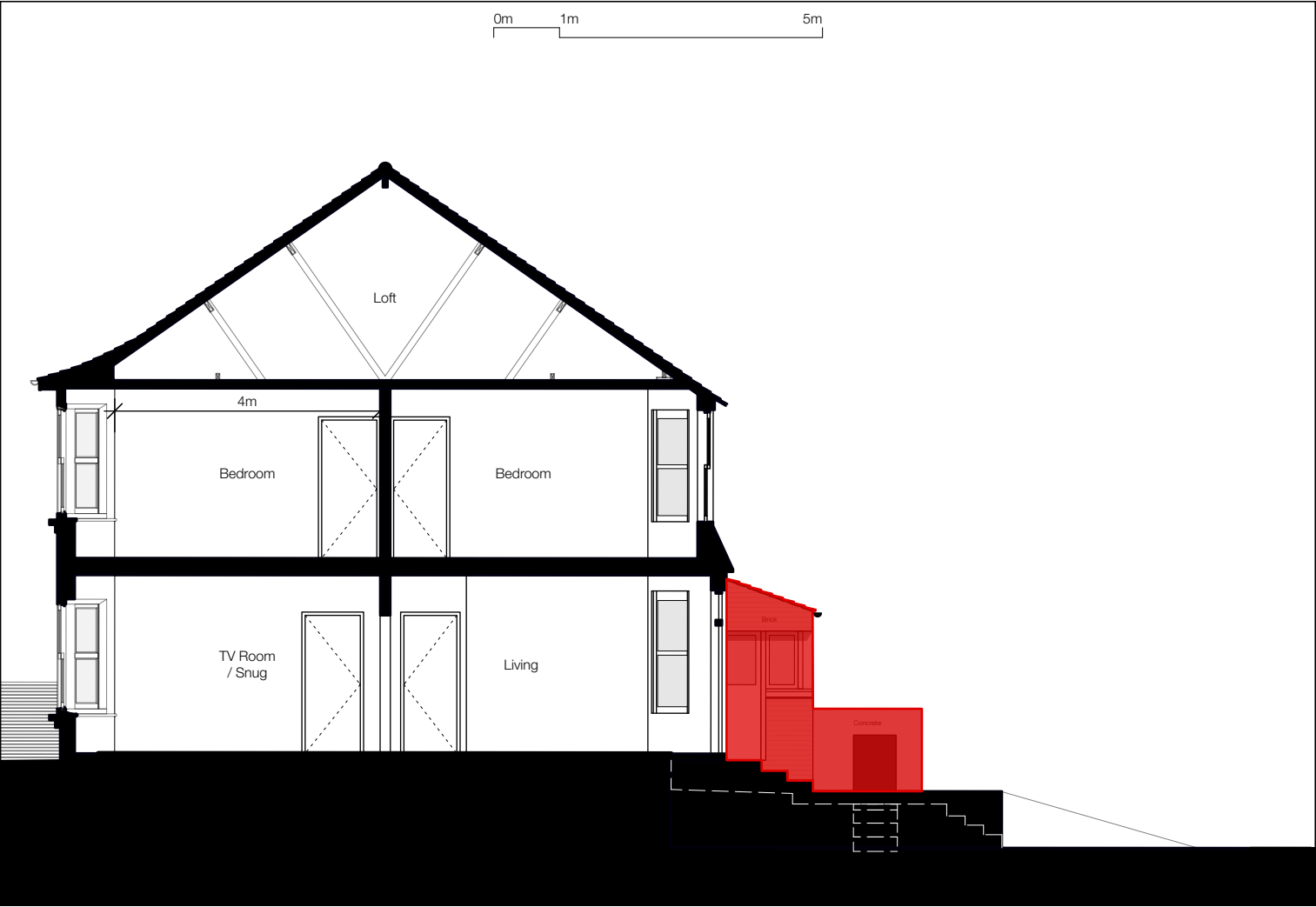
West Elevation / Section AA EXISTING
