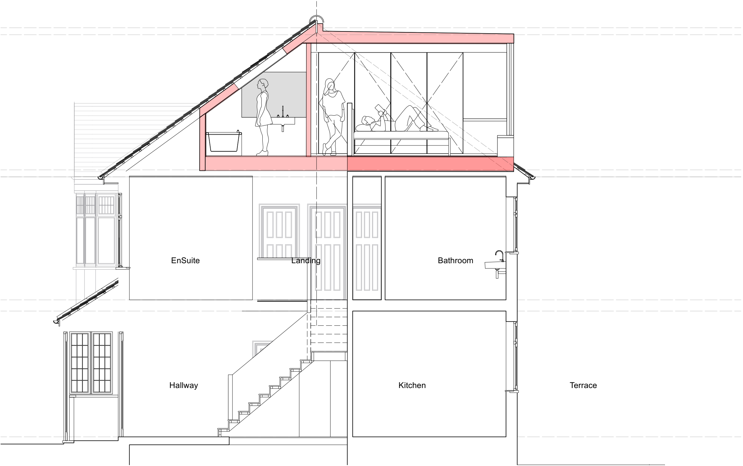
Proposed Cross Section A-A
