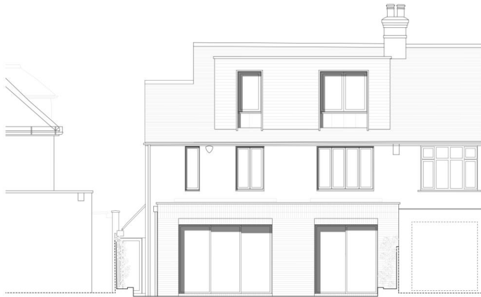
3.1 Rear elevation as proposed. The form and fenestration of the additions are informed by the size and location of existing window openings, providing a considered and cohesive appearance.
