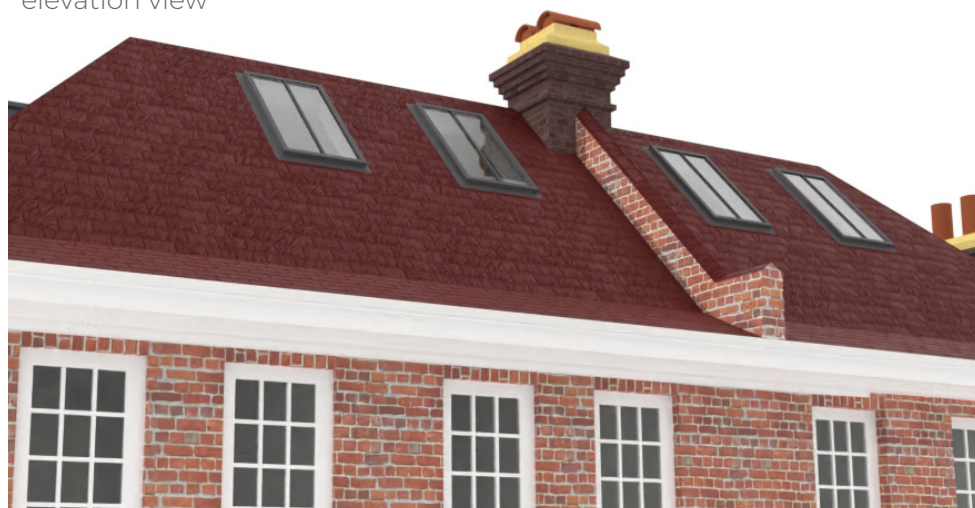
5 - Side dormer and conservation roof windows
