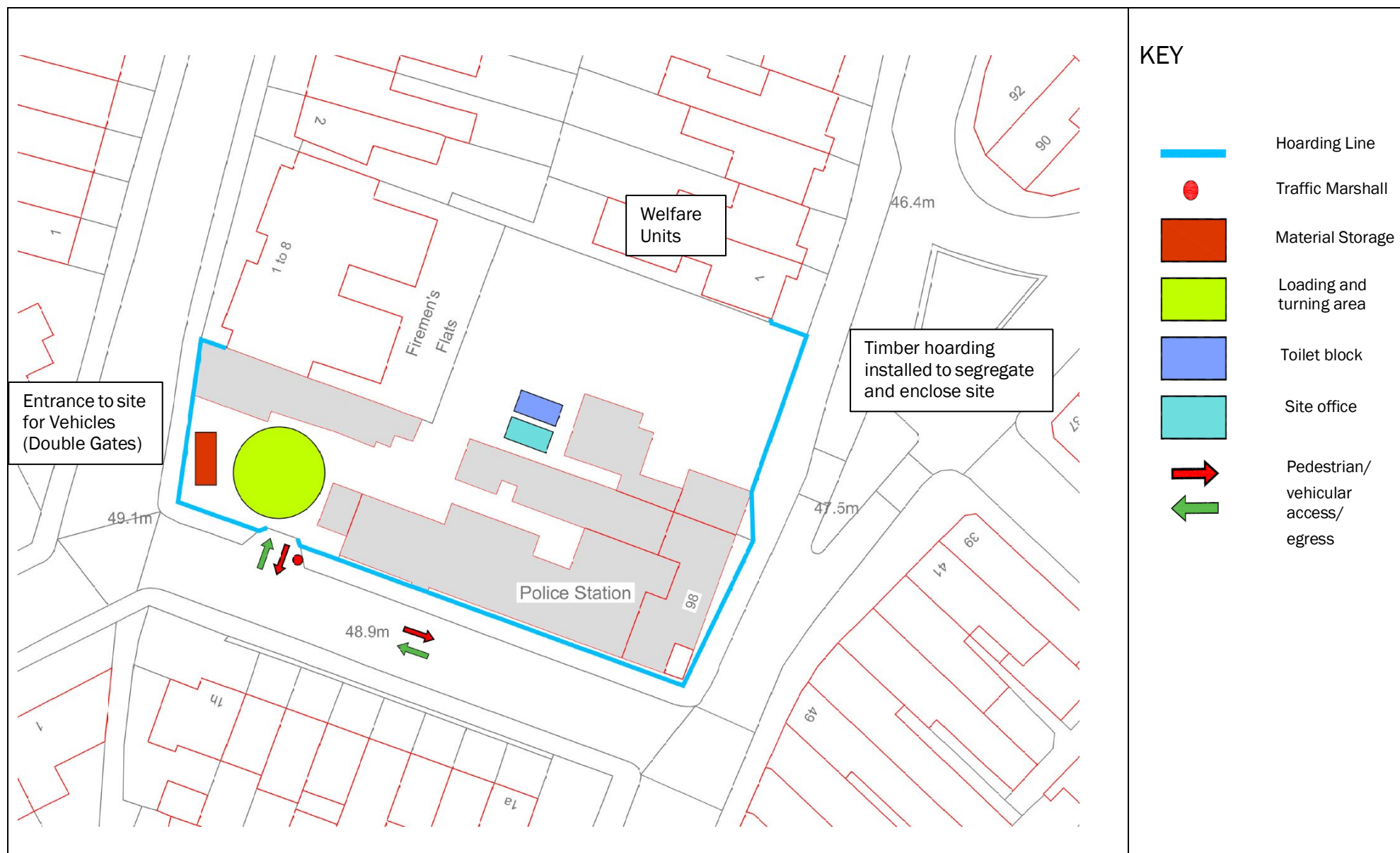
Figure 6.2: Site Map (Construction)
