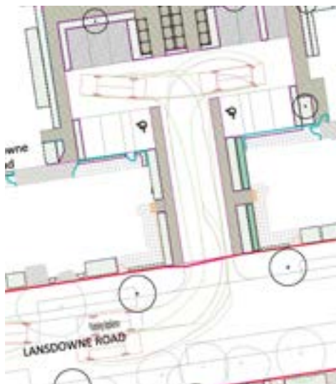
Fire Vehicle tracking for dwellings on Arundel
