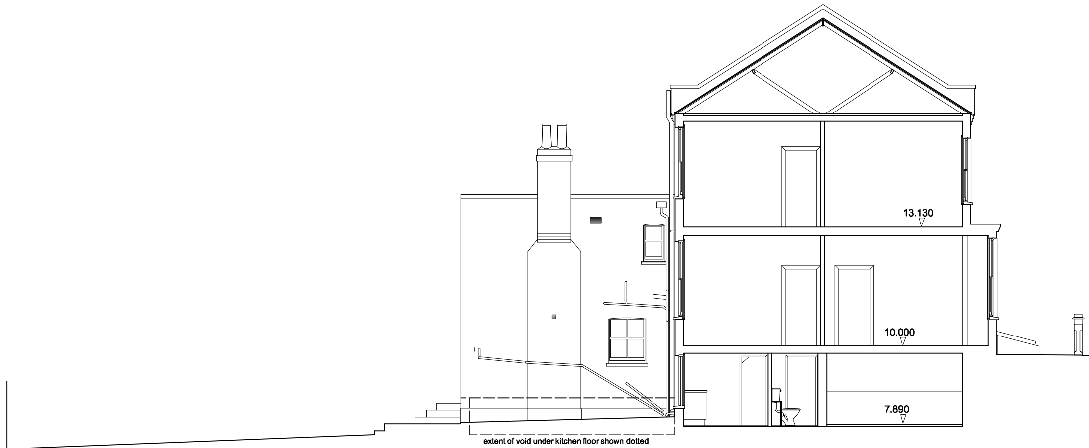
Section BB as existing
