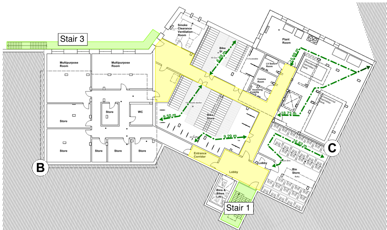
Figure 5. This corridor provides alternative escape routes from all rooms within the basement.
