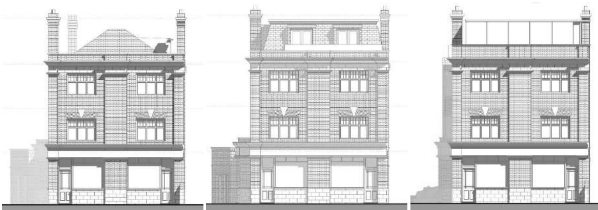
Figure 3: Pre-existing, existing and proposed front elevation
