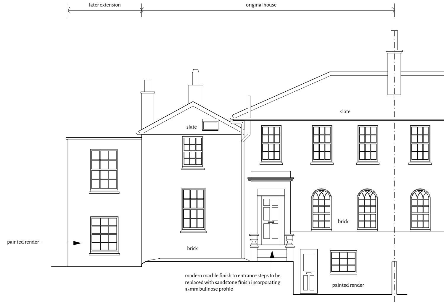
Front Elevation (north)
