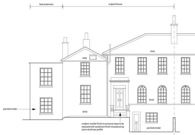
Front Elevation (north)
