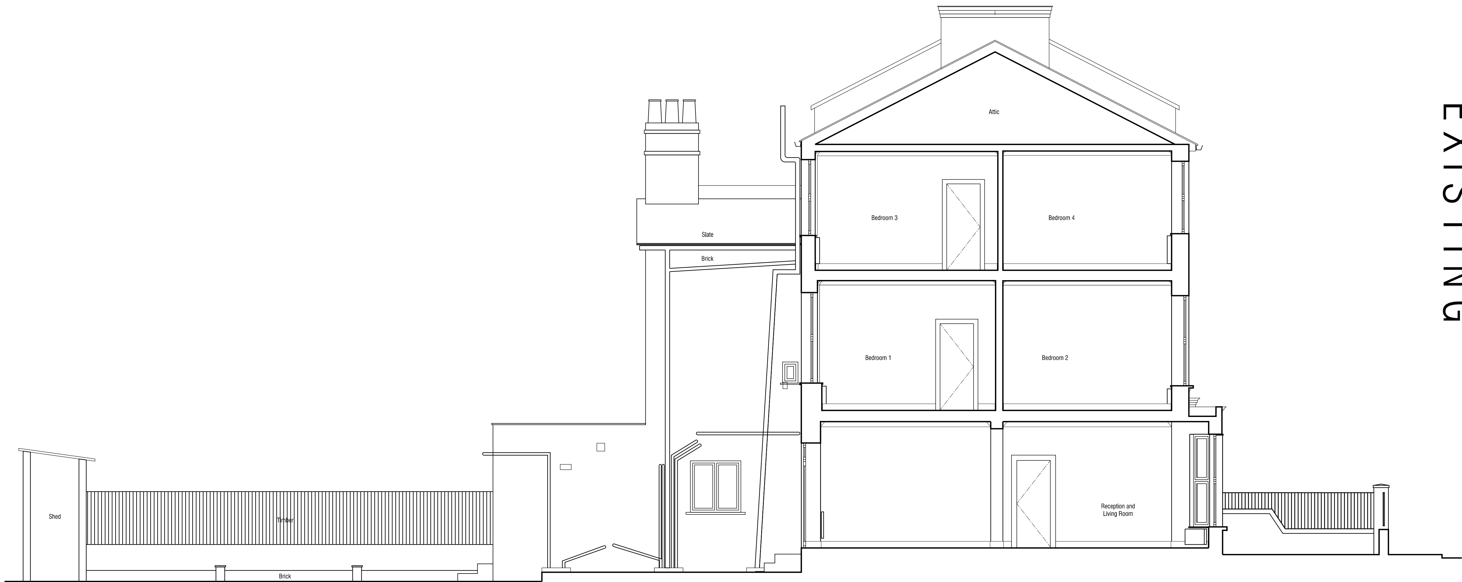
327/03/104 EXISTING SECTION AA 01 SCALE = 1:50
