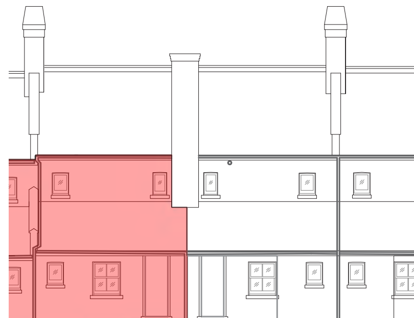
REAR ELEVATION DEMOLITION
