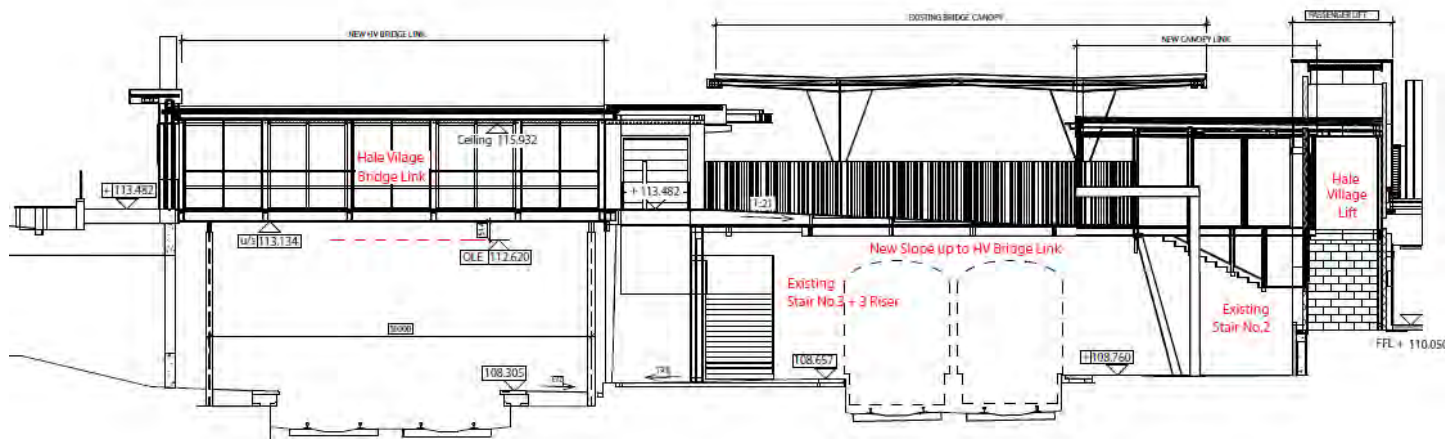
Figure 1 Cross-section drawing of the proposed link bridge between Hale Village and the existing station structure viewed from the north.
