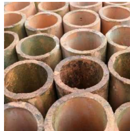
Reclaimed terracotta land drain pipes
