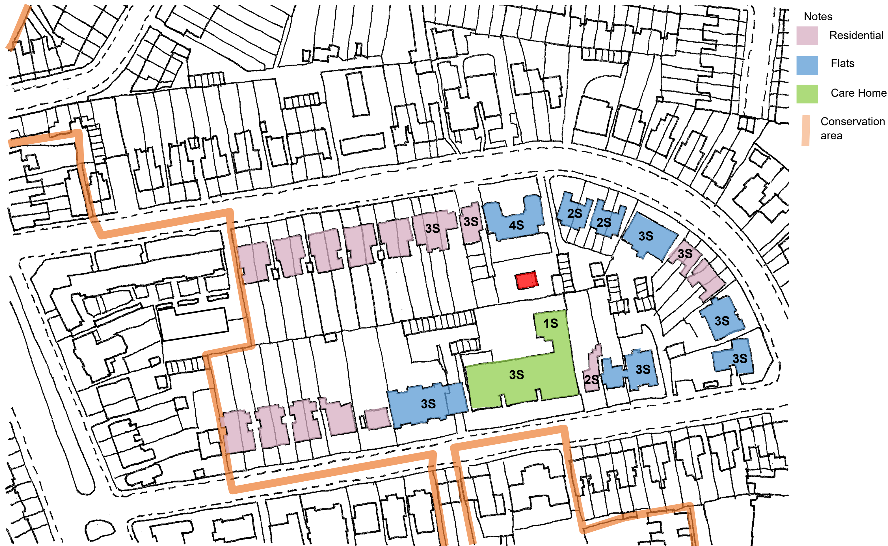
Image 15 Analysis of building around the proposed site. The majority of the surrounding buildings are three stories (3S). Orchard Cottage shown in red
