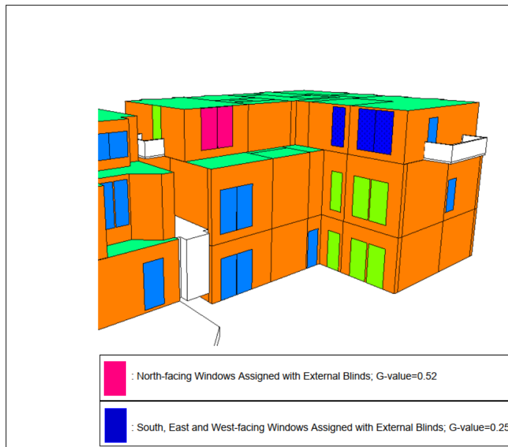
Figure 3.4: External Blinds - Block C (Northeast Elevation)
