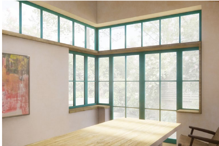
View from dining room - note high level glazing and minimal eye level glazing towards neighbours boundary
