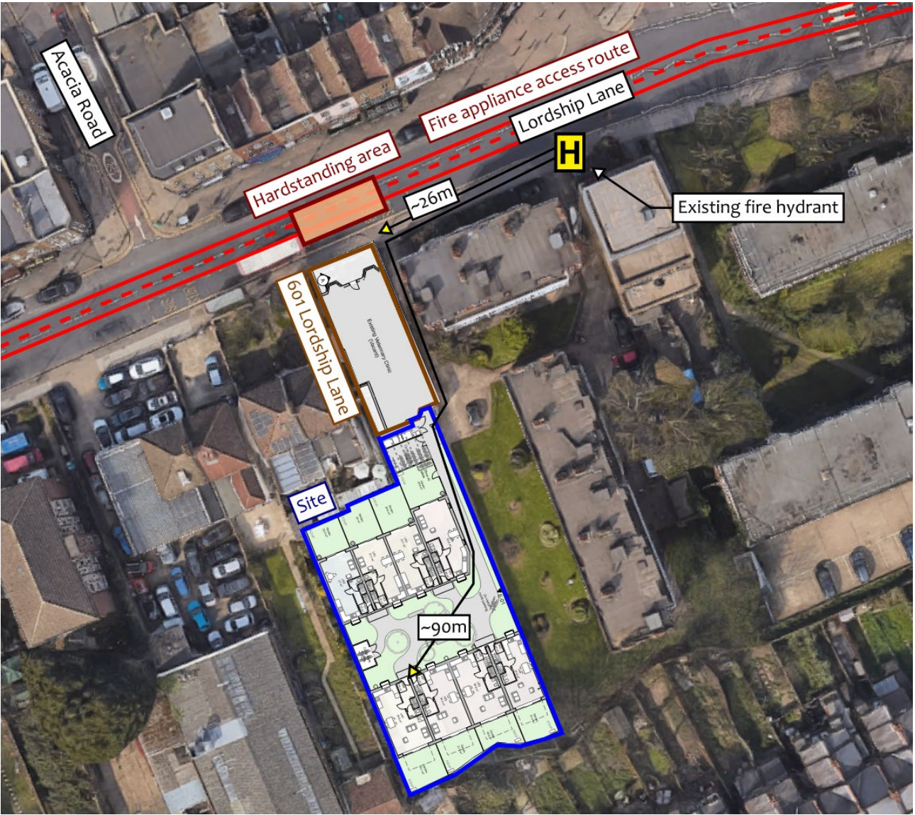
Figure 11 – Firefighting vehicle access and water supplies
