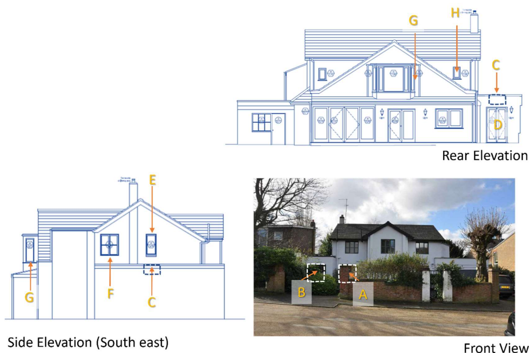
Figure 5. 6 Grange Road. Annotated figures of the windows analysed. Windows A and B cannot be seen from the front view photograph, but together with glass door D and rooflight C light a kitchen/dining area. Windows E and F directly facing the proposal light a bedroom. Windows G and H light a bedroom. Front view photo edited from Viridian photos 02 in planning application HGY/2016/3135. Rear and side elevation edited from Anne Machin Architects' drawings in planning application HGY20151698.
